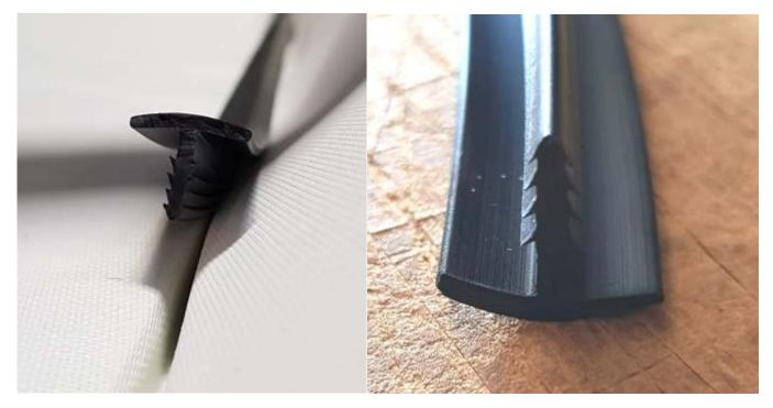
Above our brilliant new fabric insert profile. This is a 100 series PVC extrusion with 4 sets of flexible wings. A breeze to insert, easy to remove yet hard to push out under tension. Based on the snap buttons used in the automotive industry.
